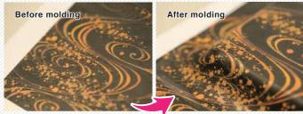
Intricate textures of decorative fine prints are retained even after molding. Furthermore, raised areas of thickly applied ink and double/triple layer printing also stay intact without cracking.
