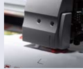
A light pointer easily adjusts the head position to the crop marks.
